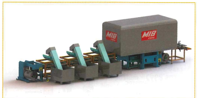
The line serves for the production of structured panels from waste
